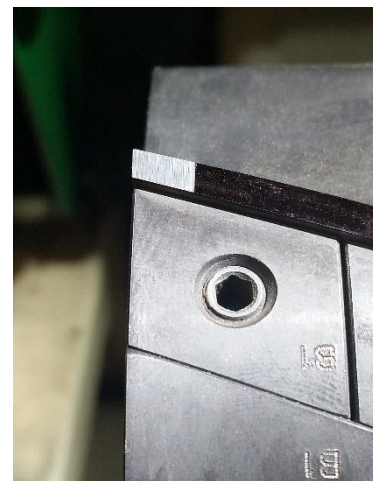
Use black marker to see the effect of sharpening
