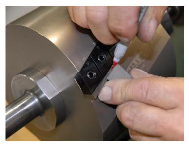
1. Mark a line on the top of the blade 1/16" (0.063) from the cutting edge.
