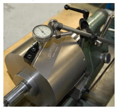
2. With the cutter mounted in a checking fixture, place a dial indicator at the cutting edge and set the indicator to zero.
