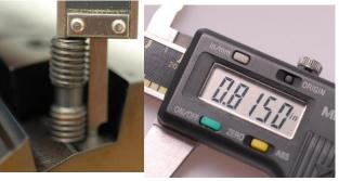
Place anti-seize on the left-hand threads of the screw. With the narrow end of the wedge on top of the screw, turn the screw clockwise 5-6 revolutions with the appropriate T-handle key. Repeat this procedure for all wedges and screws to be replaced.
